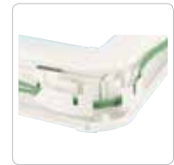
VDI accessories ensures bending radius required by the standards. Bending radius should be 8 times the diameter of cable
